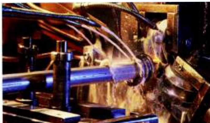
HFW induction welding in progress.
