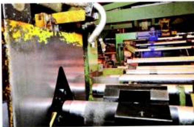
Threading machine used for threading of tubes ordered in threaded and socketed condition
