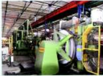
2. HR Coil inserted on the uncoiler
