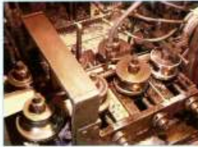
5. Formation of Tube through the rolls
