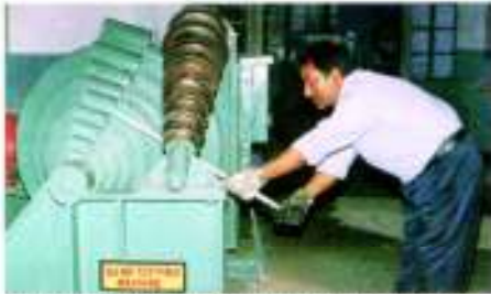
Bend testing machine used for testing bend ductility, weld quality and quality of zinc coating on the tubes
